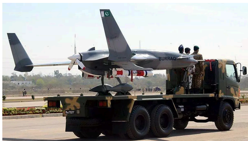
Burraq is based on Chinese designs. It features a pusher-propeller configuration, straight wings, and a V-tail. Designed primarily for precision strike missions, Burraq is equipped with laser-guided air-to-surface missiles and has been used in counterterrorism operations within Pakistan's borders Source: Millennium Post.
