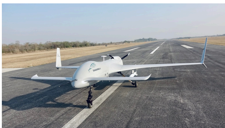
Shahpar-II is a MALE drone developed by Pakistan's Global Industrial & Defence Solutions (GIDS) for intelligence, surveillance, and precision strike missions. It features a pusher-propeller configuration, high-mounted straight wings, and a V-tail. The drone is equipped with electro-optical sensors and can carry guided air-to-surface munitions. Shahpar-II has an endurance of over 14 hours and supports both day and night operations. Source: Aaj Tak
