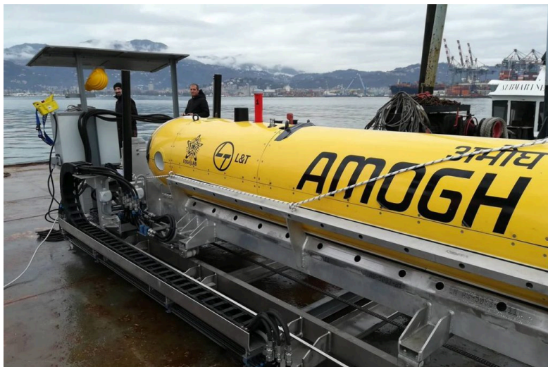
The Amogh is a deep-water Autonomous Underwater Vehicle (AUV) developed by L&T Precision Engineering and Systems (in collaboration with EdgeLab, Italy), specifically designed for modern hydrographic surveys. It meets IHO S-44 special order standards, delivering high-quality, high-resolution data with excellent positional accuracy. Source: Indian Aerospace and Defense Bulletin
