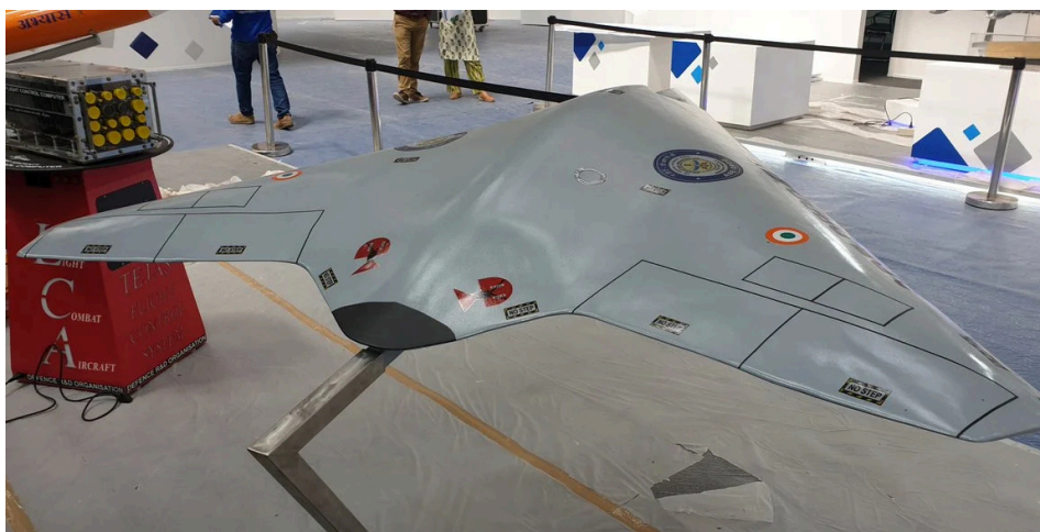
The Ghatak is an autonomous, jet-powered, stealth unmanned combat air vehicle (UCAV) being developed by the Aeronautical Development Establishment (ADE), DRDO. Source: www.defense.in
